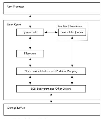
Figure 4-2: Kernel schematic for disk access
