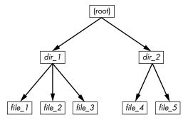
Figure 4-9: User-level representation of a filesystem
