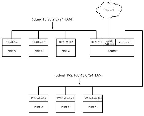
Figure 9-5: Two subnets joined with a router
