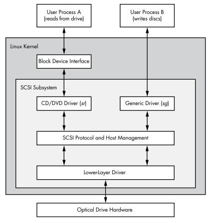
Figure 3-3: Optical device driver schematic
