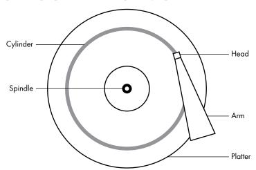
Figure 4-3: Top-down view of a hard disk
