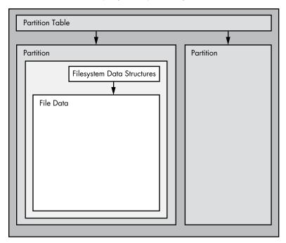
Figure 4-1: Typical Linux disk schematic
