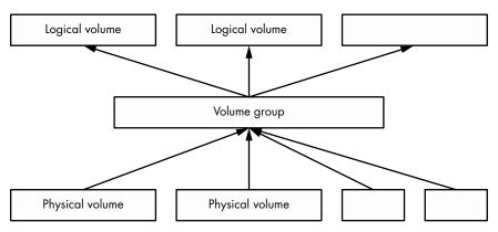
Figure 4-4: How PVs and logical volumes fit together in a volume group
