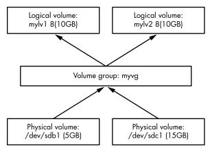
Figure 4-5: Constructing a logical volume system
