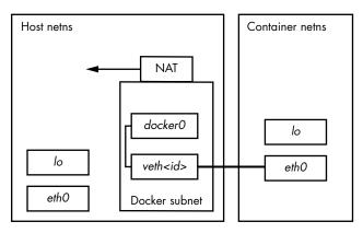
Figure 17-1: Bridge network in Docker. The thick link represents the virtual interface pair bond.
