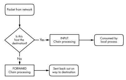
Figure 9-6: Chain-processing sequence for incoming packets from a network
