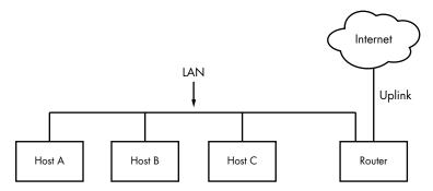
Figure 9-1: A typical local area network with a router that provides internet access
