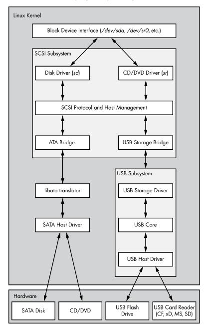
Figure 3-2: Linux SCSI subsystem schematic
